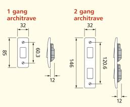
Sectional drawings show the furthest projections from the back of the frontplate (wall surface).
